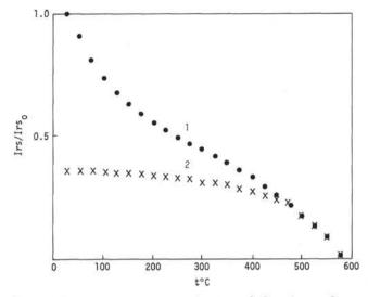
Figure 4b. Remanence magnetization of class 1 samples as a function of temperature for progressive heating and then for progressive cooling.
