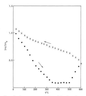
Figure 4h. Remanence magnetization of class 4 samples as a function of temperature for progressive heating and then for progressive cooling.
