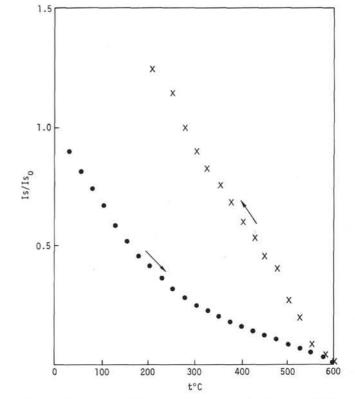
Figure 4i. A plot of the saturation magnetization in a 5000oe field as a function of progressive and regressive temperature for class 5 samples. Note the differences between the heating curve and the cooling curve due to mineral alteration during heating.
