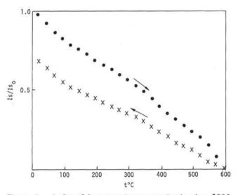
Figure 4c. A plot of the saturation magnetization in a 5000oe field as a function of progressive and regressive temperature for class 2 samples. Note the differences between the heating curve and the cooling curve due to mineral alteration during heating.
