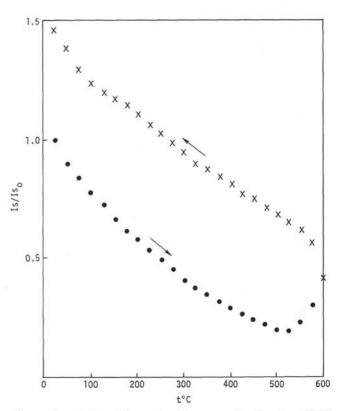
Figure 4g. A plot of the saturation magnetization in a 5000oe field as a function of progressive and regressive temperature for class 4 samples. Note the differences between the heating curve and the cooling curve due to mineral alteration during heating.
