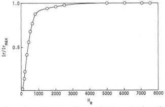
Figure 2. A plot typical of normal (more common) samples of Ir/Ir<sub>max</sub>. as a function of the magnetic field. Note the positions of Hes and He's.
