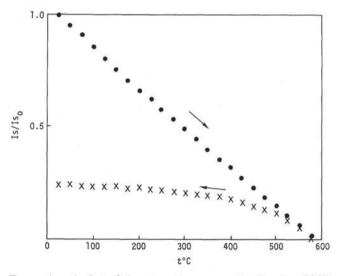
Figure 4a. A plot of the saturation magnetization in a 5000 oe field as a function of progressive and regressive temperature for class 1 samples. Note the difference between the heating curve and the cooling curve due to mineral alteration during heating.
