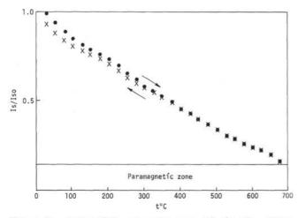
Figure 4e. A plot of the saturation magnetization in a 5000oe field as a function of progressive and regressive temperature for class 3 samples. Note the differences between the heating curve and the cooling curve due to mineral alteration during heating.
