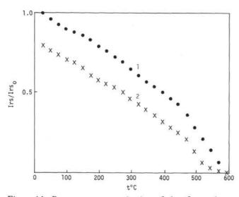
Figure 4d. Remanence magnetization of class 2 samples as a function of temperature for progressive heating then for progressive cooling.
