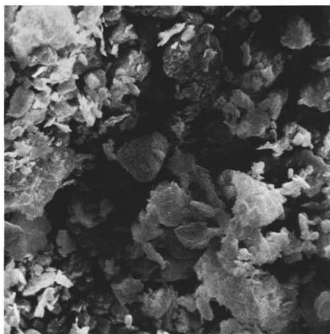
Figure 7. Laminites from the upper Messinian of the Balearic Basin (DSDP Site 124, Core 7, Section 1, 79-81 cm). Unlike the Messinian laminites cored at Site 372, here the clear laminae (A) do not correspond to coccolith blooms. They do not differ markedly in texture from the gray sandy layers (B).
