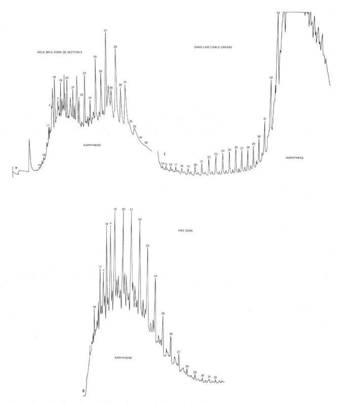
Figure 1e-g. Gas chromatograms of the saturate hydrocarbon fractions.
