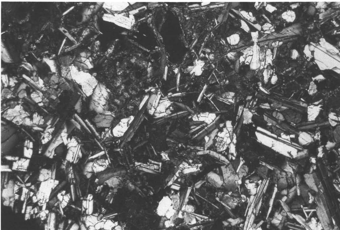
Figure 39. Photomicrograph of complex intergrown plagioclase and clinopyroxene with very little interstitial mesostasis; Sample 135-835-7R-2, 89-93 cm, Piece 5; field of view = 3 mm, crossed polarized light.
