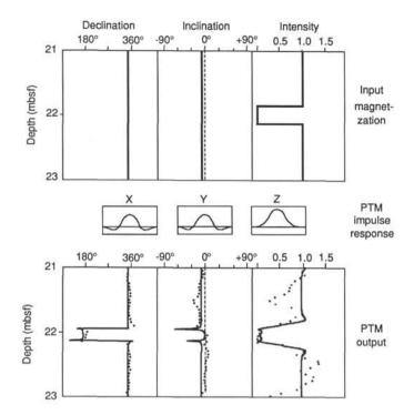
Figure 3. Pass-through magnetometer (PTM) response to a narrow interval of low intensity that gives rise to an apparent reversal of polarity. Solid lines in lower panels indicate calculated magnetometer output for a gap within a region of uniform magnetization. The configuration modeled very closely matches the observed magnetometer output (discrete points) from Core 115-710A-3H where a 25-cm section had been removed for geochemical analysis.
