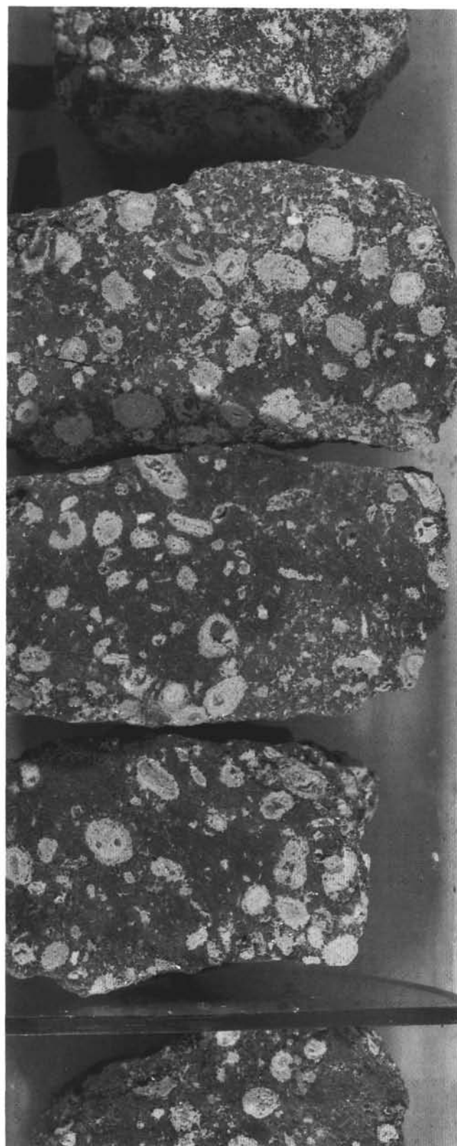
Plate 1. Stages in the dolomitization process. 1. Brown sucrosic dolomitic groundmass and scattered unaltered calcitic white oncoid bioclasts (core photograph Section 143-866A-159R-1, 20-34 cm). 2. Similar to 1, but with calcitic bioclast dissolution leaving prominent moldic porosity. Some parts of this core contain no original calcitic bioclasts (core photograph Section 143-866A-159R-3, 70-84 cm).
