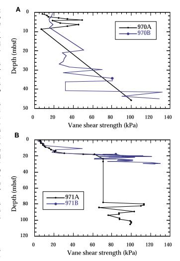
Figure 6. Summary of results from vane shear strength obtained routinely during Leg 160 from (**A**) Site 970 (Milano) and (**B**) Site 971 (Napoli).
