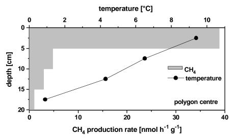
Fig. 9.8 Vertical profile of *in situ* methane production and soil temperature for a permafrost soil of the polygon center.
