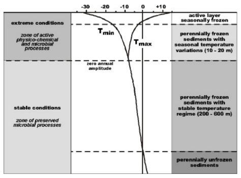
Fig. 9.1 Scheme of temperature amplitude in permafrost sediments (according to French [4], modified).
