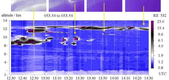
Data of clouds and aerosol measured by Marl in Lindenberg on August, 8<sup>th</sup> 2003. The upper pictures show cirrus cloud and contrails photographed by the cloud camera. The clouds are identified in the lidar data. Thus, the height and optical properties like the optical depth, the color index and the depolarization can be determined. Based on the closest radiosonde data, the relative humidity at which the clouds occur can be estimated.
