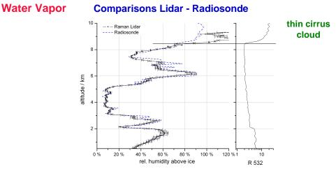
Comparison of lidar (black) and radiosonde (blue) measurements of water vapor (in terms of the relative humidity). The sonde was started at 22:45 of June 17 2003 and reached 10 km about half an hour later. The graph at the right hand side shows the backscatter ratio profile determined by the lidar at the same time (22:53 - 23:05, 20,000 shots). Up to the thin cirrus cloud in 8.5 km altitude the measurements by the radiosonde and lidar agree very well.
