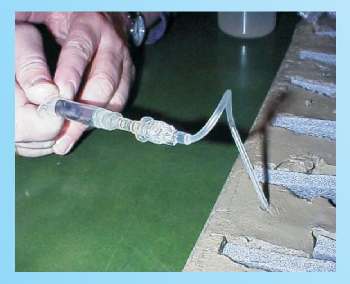
Fig. 2: Rhizon pore water sampling in marine sediment cores, to our knowledge the first attempt to collect pore water samples from marine sediments using rhizon soil moisture samplers..
