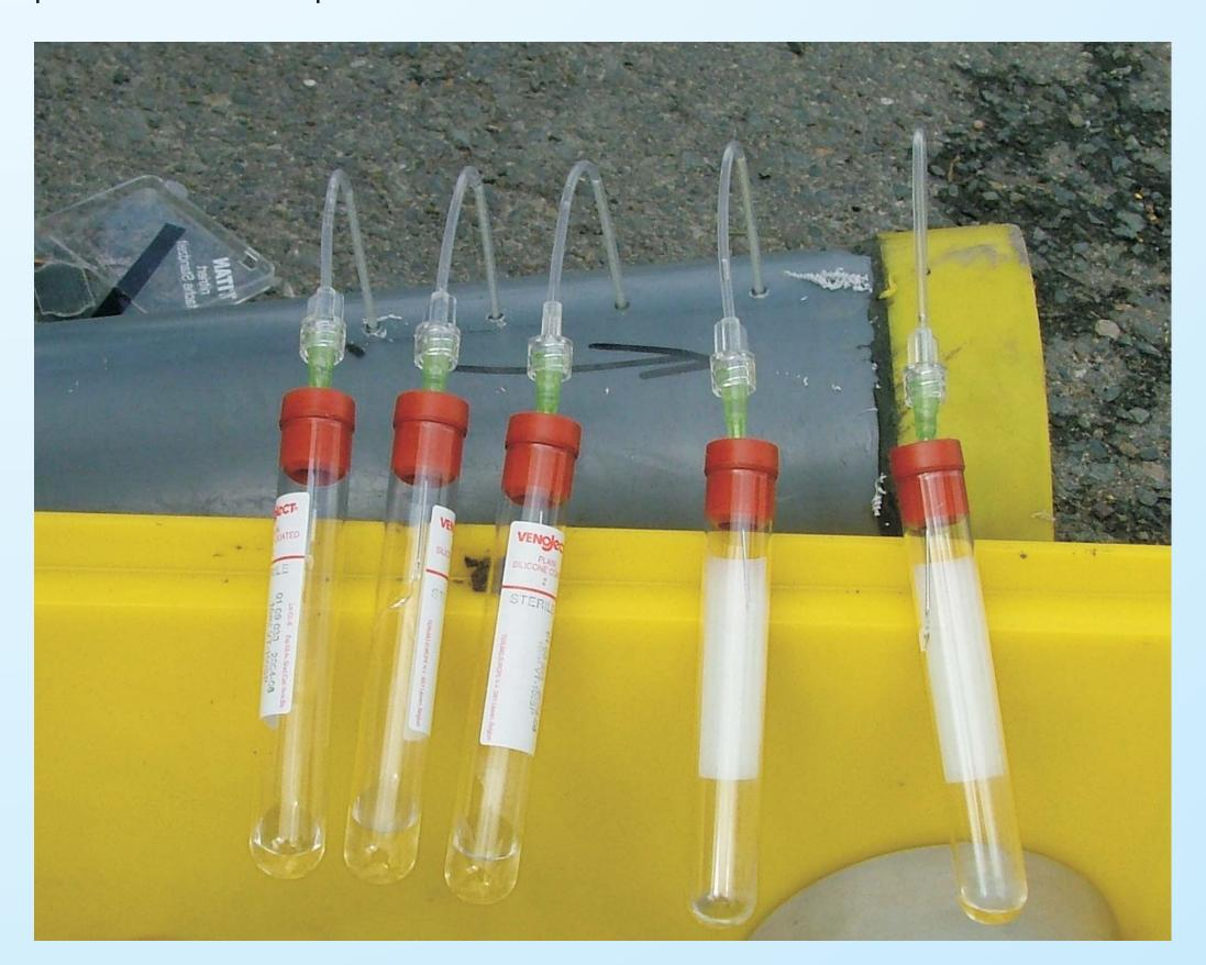
Fig. 7: Pore water sampling from a core liner using Rhizon samplers attached to a needle and blank vacutubes. For special purposes also preloaded vacutubes may be used
