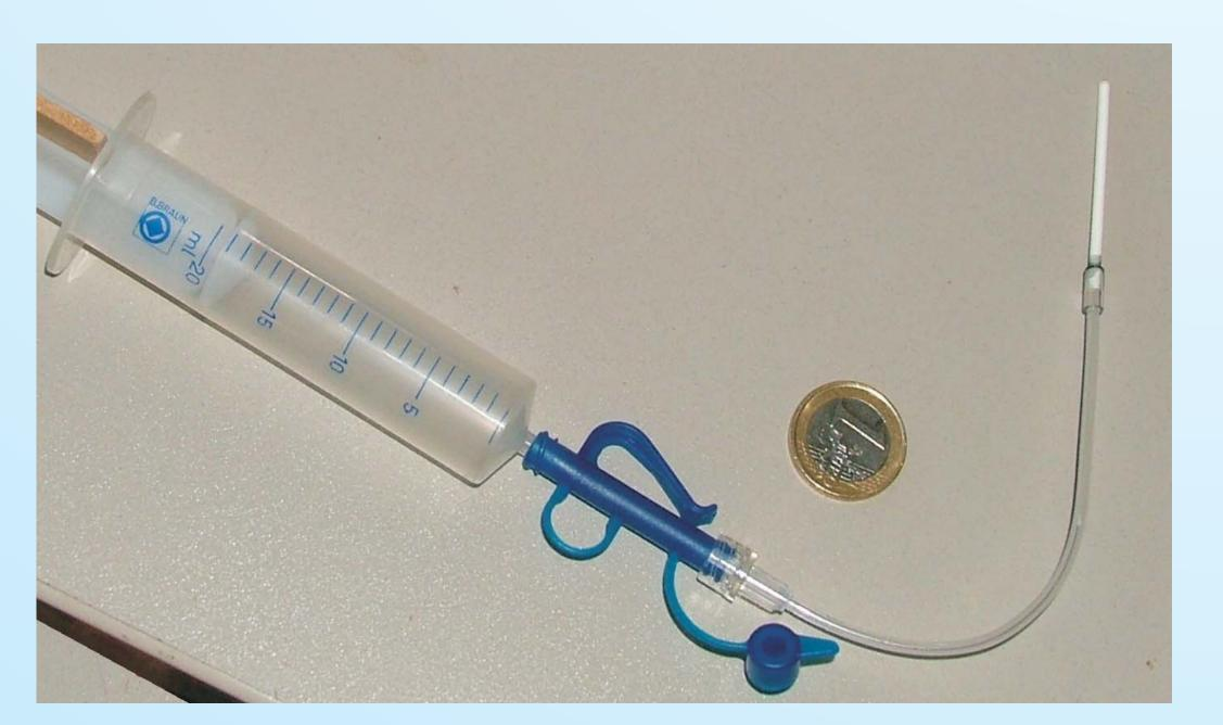
Fig. 5: Rhizon Core Solution Sampler connected to a 20 mL disposable syringe. Vacuum is simply applied by pulling the plunger and keeping it in place with a spacer.
