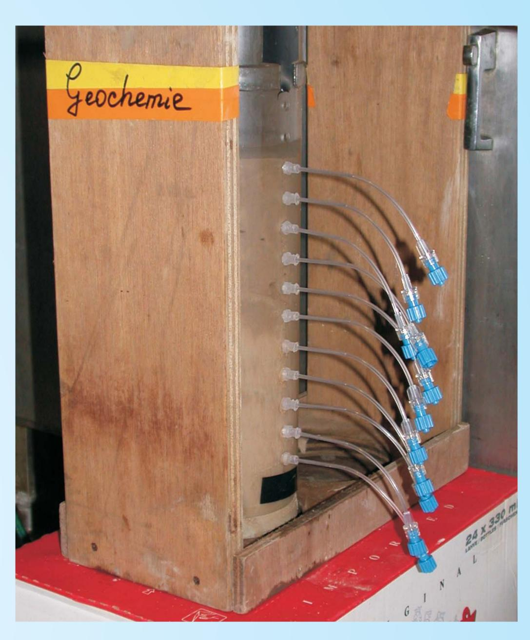
Fig. 8: Porewater sampling from MUCs. Multicorer liner tube on a Polarstern Cruise with rhizons installed through predrilled holes in the liner wall. Sampler connectors are sealed by blue caps until syringes are attached. Vertical distance of sampling points is 2 cm.
