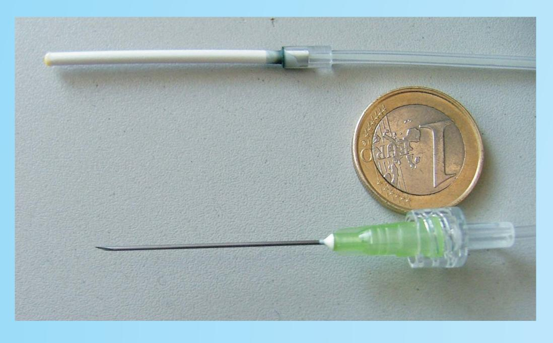
Fig. 1: Rhizon Core Solution Sampler, 50mm length, 2.5mm diameter (Rhizosphere Research Products, Wageningen NL). The hydrophilic microporous tube (white) is supported by a nylon wire. The sampler is connected to Tygon tubing.
