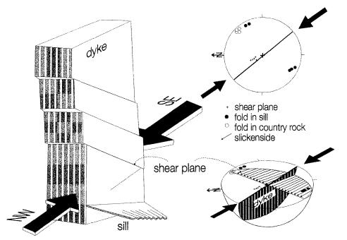
**Fig. 8:** Block diagram of a compressively deformed dyke (about 2 m thick) in the Cretaceous dyke swarm in northernmost Greenland (Lockwood Island) (for location see Fig. 7).
