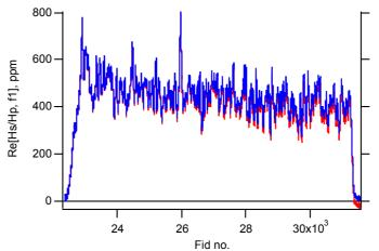
**Figure 4:** Typical profile of inphase component of  $f_1$  (3.6 kHz) showing original (red, stippled) and drift-corrected trace (blue, solid). February 23,  $2^{nd}$  flight, file 200302231204\*.
