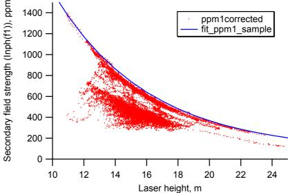
**Figure 5:**  $F_1$  Inphase signal versus system height above the ice surface for the example for the April 11 flight, which crossed large stretches of thin ice and some open water. The exponential fit is performed only for open water sampling points.
