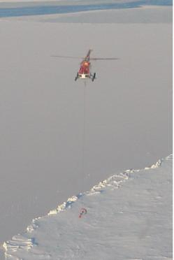
Figure 3: EM bird in operation.
