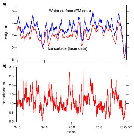
Figure 6: Profiles of bird height above the water (blue) and ice (red) surface (a) and ice thickness (b) derived by subtracting both curves in a.
