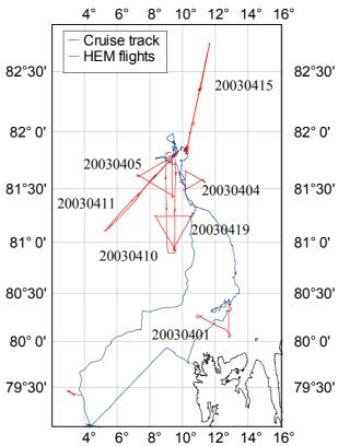
**Figure 1**: Cruise track of RV Polarstern during the first GreenICE field campaign in 2003 (blue). Red lines show thickness profiles surveyed by helicopter electromagnetic (HEM) sounding.
