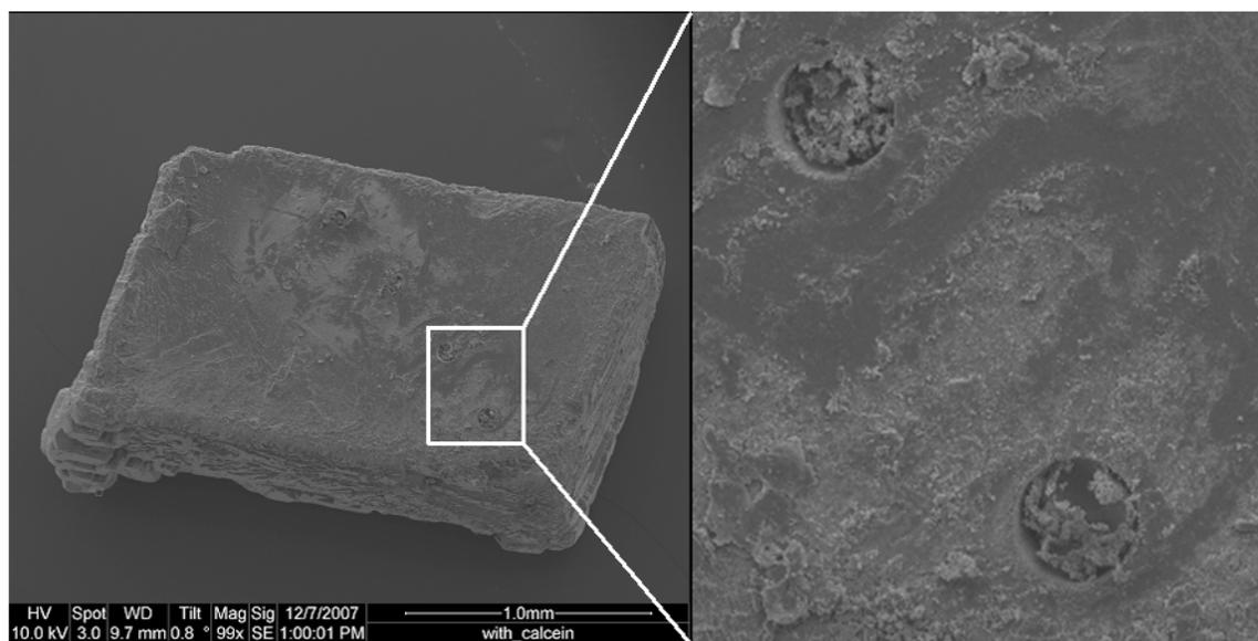
**Figure 3.** (left) SEM image of an inorganically precipitated calcium carbonate crystal (precipitated in the presence of the fluorescent compound calcein). (right) Ablation craters performed with the LA-ICP-MS.
