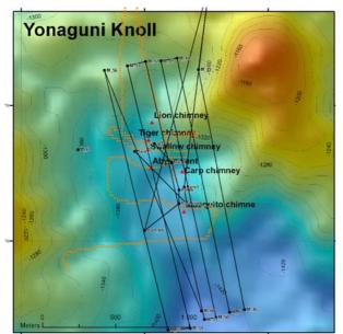
Fig. 6.7: Parasound survey #1(st. 12) tracklines covering all chimneys centred around Abyss
