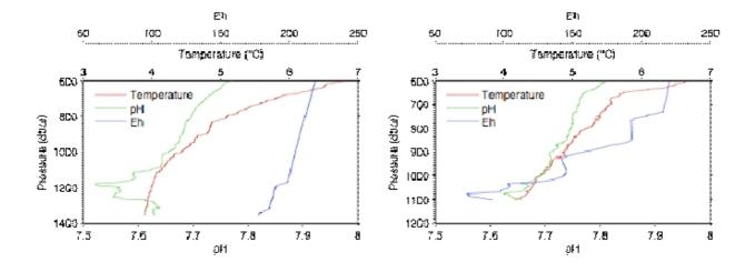
Fig. 6.12: Vertical profiles of temperature, pH and Eh uncalibrated data at two different locations in the Yonaguni Knoll IV area: One close to the known vents (station 68, left) and one northeastward of the vents (station 57, right)
