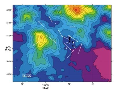
Fig. 6.14: Bottom currents from LADCP measurements; shown are the mean velocities in the lower 100 m of the water column
