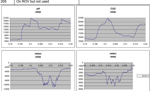
Fig. 6.20: Sensor measurements recorded above a  $CO_2$  seep. pH signals increase with decreasing pH;  $CO_2$ signals increase with increasing  $CO_2$ , and redox signals decrease with decreasing redox state. The time is given as fraction of the day, normally the handheld was placed for ca 10 minutes
