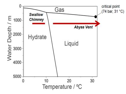
Fig. 6.22: Phase diagram of  $CO_2$  in seawater (after Duan and Sun, 2006). Indicated in red are the p,T conditions at the 2 primary investigation sites in the Yonaguni Knoll IV area, Swallow Chimney and Abyss Vent. Due to the prevailing porewater and bottomwater temperatures,  $CO_2$  hydrates are only stable in the surface sediments of Swallow Chimney, whereas at Abyss Vent liquid and supercritical  $CO_2$  dominate
