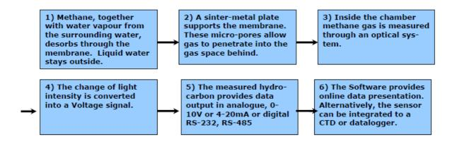
Fig. 5.7: Work flow of the *HYDOC*-  $CH_4$  measuring process. The principle of this sequence remains the same for measuring  $CO_2$  instead of methane
