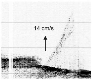
Fig. 6.5: 18 kHz water column reflection recorded by *PARADIGMA*. Data pattern indicates a rising reflector
