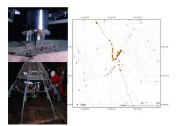
Fig. 6.35: Videoguided transects with the TV MUC (S-N) or ROV (SW-NE). A microprofiler was installed to measure  $CO_2$  and pH during the visual monitoring of megafauna distribution
