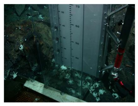
Fig. 5.6: Bubble imaging box at the seafloor above a  $CO_2/CH_4$  droplet emitting site. The front is positioned on the porch of the ROV, a gas sampler is attached on the right side of the frame
