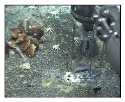
Fig. 5.2: The handheld is placed above a  $CO_2$  vent to record temperature, pH,  $CO_2$  and redox effects
