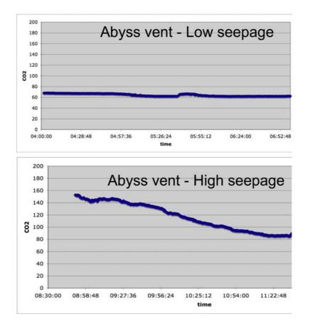
Fig. 6.32: Measurements of  $CO_2$  concentrations over time in the benthic chamber deployed at two sites close to Abyss vent with high and low seepage activities. Note that smaller signals means higher  $CO_2$ concentrations
