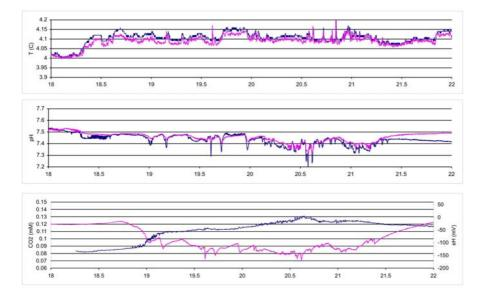
Fig. 6.29: pH and  $CO_2$  variations in the Yonaguni basin. For the transect see Fig. 6.30. The y-axis is UTC time of the transect. The seep zone is reached at 18:30, and left at 21:15
