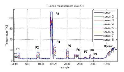
Fig. 6.26: Temperature data of P1-P9 gathered during dive 201 including the subsequent water column upcast
