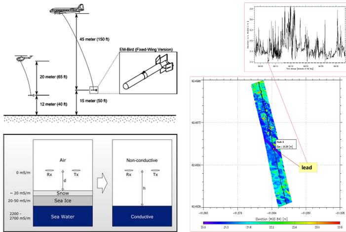
**Left:** Sketch of airborne sea ice thickness measurements with electromagnetic induction sounding based on 1D assumption: Electrical conductivity of sea ice negligible and level sea ice within footprint. Sea ice thickness is derived from the difference between sea ice/snow surface (detected by laser altimeter measurements) and the sea ice-ocean interface (derived from EM data).
