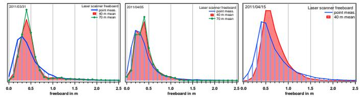
Laser scanner freeboard data are averaged over the footprint-areas of the EM-Bird thickness measurements (40 m, red) and the ICESat footprint (70 m, green).
