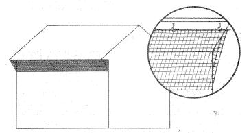
Figure 2: Plastic netting or wire mesh can be attached to a building from the outside edge of eave and angled back to the wood siding to exclude woodpeckers. Insert shows one method of attachment using hooks and wooden dowels. (Adapted from Woodpeckers [1983]), by Rex E. Marsh in R. M. Timm (ed.), Prevention and Control of Wildlife Damage, Cooperative Extension Service, University of Nebraska, Lincoln.
