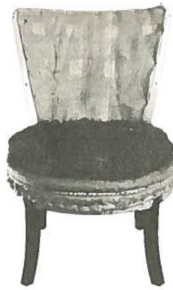
Fig. 57—Moss padding sewed in place. Seat ready for cotton padding. Back webbing covered with burlap.
