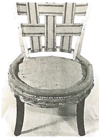
Fig. 56—The fireside chair. Webbing and springs in place, covered with burlap and hard edge roll put on.
