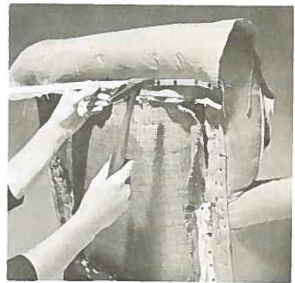
Fig. 53—Blind tacking outside back at top.
