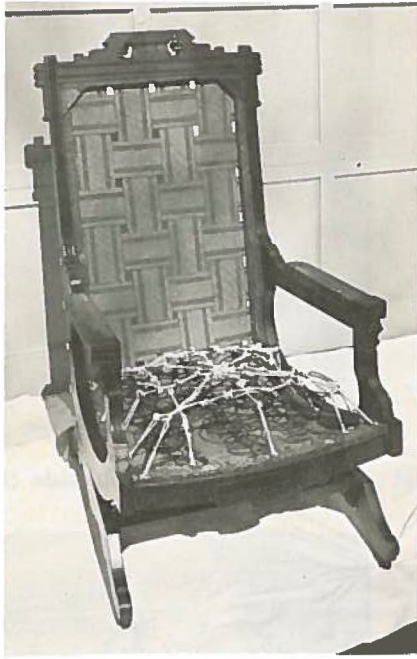
Fig. 62—The platform rocker with webbing in place and springs completely tied for a flat seat.
