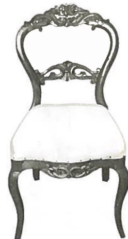
Fig. 61—Cotton padding over burlap is covered with muslin. Seat is ready for outside covering.
