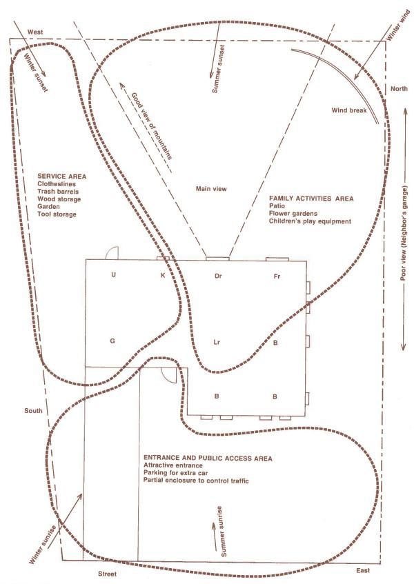
Figure 4. Completed analysis plan.
