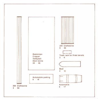
Figure 8. Scale outlines of auto, boat, trash barrels, etc. to be cut out and placed on trial plan for determining space requirements.
