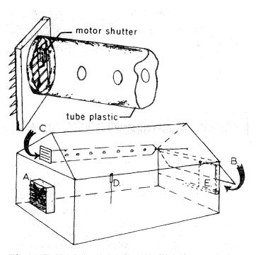
Figure 1. Components of a ventilated greenhouse.
