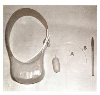
Fig. 1. Transceiver neck-collar, left, and heart-pulse transmitter, right, used to monitor heart-rates of deer. Two stainless steel electrodes exit from transmitter within a protective teflon plastic tube and surface outside the tube (points A and B) to contact animal tissue. (Photo by F. Waugh)
