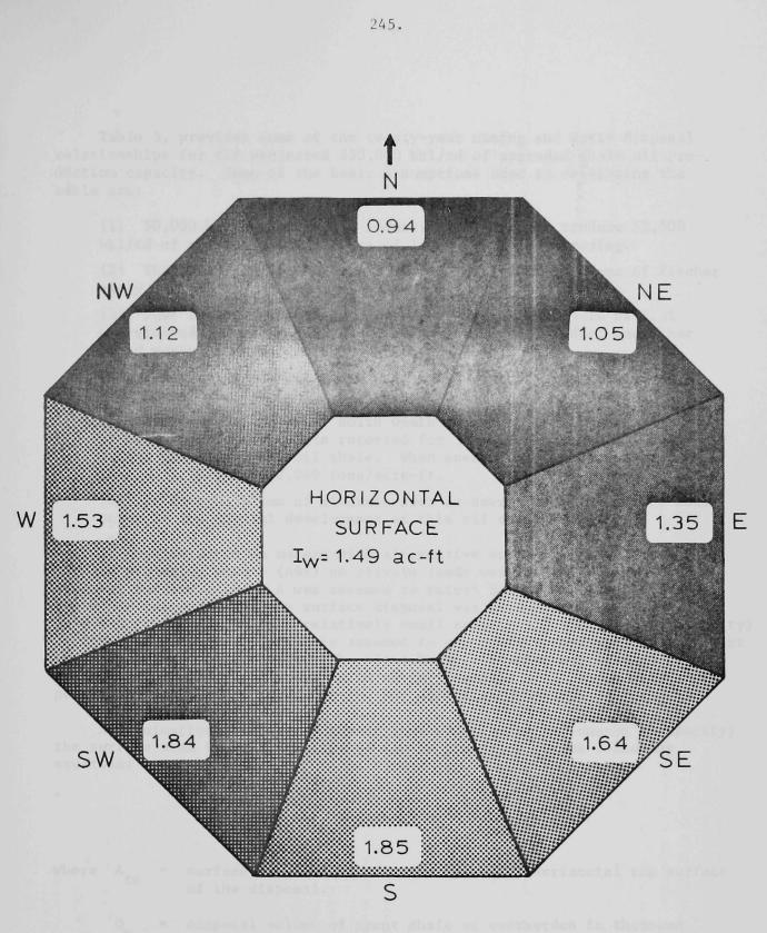
Figure 1. Estimated irrigation water required (Acre-feet) for full season irrigation on the horizontal surface and 25% slope facings of revegetation areas at 7,000 ft.
