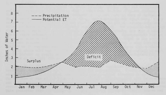
Figure 2. Water balance for the Piceance Basin at 8000 feet elevation.
