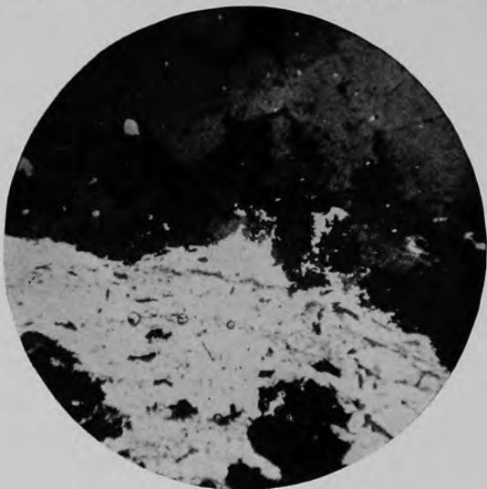
B.—PHOTOMICROGRAPH OF ORE FROM GARFIELD MINE Dark gray mineral is pyrite; black minerals are galena and zinc blende; light mineral is chlorite. Ordinary light; x 14.
