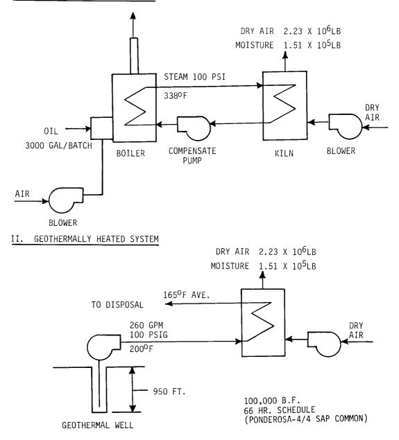
Figure 13. Conventional and Geothermal Lumber Kiln Driers (from V.T.N.-C.S.L., 1977).
