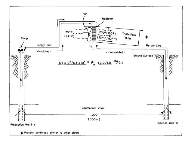
Figure 12. Rotary Drum Alfalfa Dryer (from Lienau, 1979).
