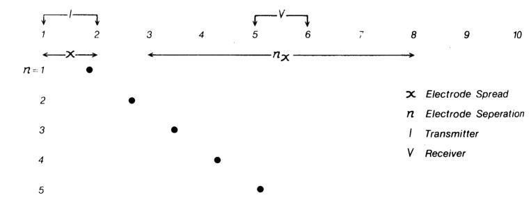
Figure 23. Typical dipole-dipole array (from J. Combs, 1980).
