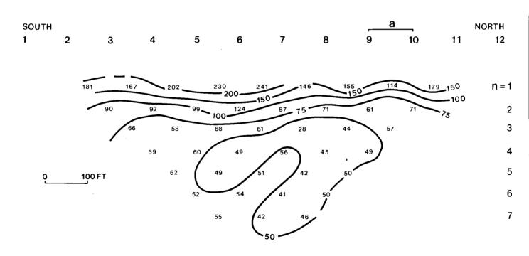
Figure 8. Dipole-Dipole Pseudosection Line D: This north-south line located west of the warm spring also crosses Cement Creek. It is 1,200 ft (366 m) in length and shows similar characteristics as line C with resistivity values decreasing with depth. These measurements indicate that the alluvium along Cement Creek is quite thick. No faulting is apparent. LENGTH: 1200 ft | 366 m) SEPARATION: n Value DATE: 6/12/81 TYPE: Dipole - Dipole SPREAD: 0 = 100 ft RESISTIVITY: In ohm meters
