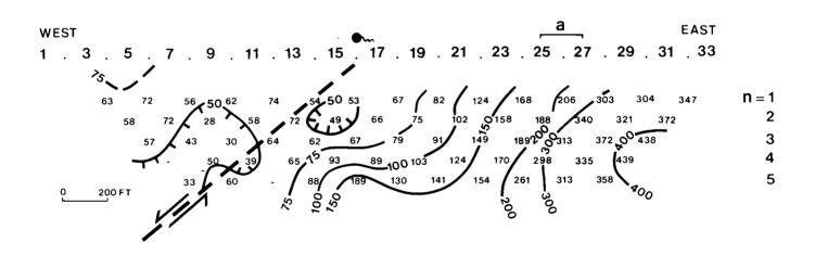
Figure 6. Dipole-Dipole Pseudosection Line B: This northeast trending line passes through the warm spring. A distinct low resistivity zone was mapped between stations 7 through 16 in the vicinity of the warm spring. The values in this zone are as low as 28 ohm-meters, which is quite similar to the low zone on line A and shows good alignment with the north-south fault that passes just east of the spring. Resistivity values increase dramatically to the east due to lithologic changes.
