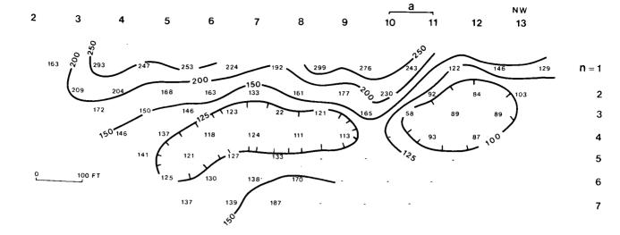
Figure 9. Dipole-Dipole Pseudosection Line E: This resistivity line trends in a northwest-southeast direction and is approximately 1,500 ft (457 m) in length. No evidence of faulting was noted. However, the contact between the alluvium of Cement Creek and the underlying bedrock is well illustrated by an increase of resistivity values at stations 6 through 8.
