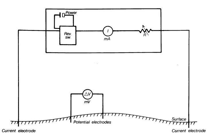
Figure 18. Schematic diagram for resistivity (from J. Combs, 1980).
