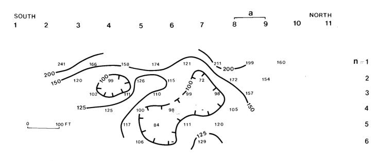
Figure 7. Dipole-Dipole Pseudosection Line C: This 1,100 ft (335 m) north-south line located east of the warm springs crosses Cement Creek. Resistivity measurements were affected by the water saturated alluvium along the creek. The near surface values are much higher than the deeper values which is probably due to water saturated aluvium. From the examination of the data no faulting was apparent.
