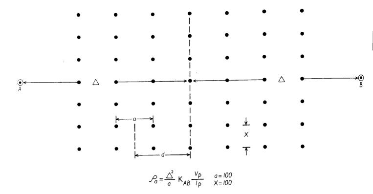
Figure 11. Plan view of the gradient array, or AB rectangle array. The rectangular area between distant, fixed current electrodes is traversed by a pair of potential measuring electrodes. Although the array factor K<sub>AB</sub> is near unity, it is a variable.
