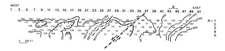
Figure 10. Dipole-Dipole Pseudosection Line F: This 5,300 ft (1.62 km) northeast trending line parallels the Cement Creek road. Resistivity measurements indicate similar characteristics with line A. A deep seated low resistivity zone was noted between stations 26 and 38 where the line crossed the north-south fault. This zone aligns itself well with the same fault illustrated on lines A and B. The resistivity values increase rapidly to the northeast, indicating a lithologic change in the bedrock.
