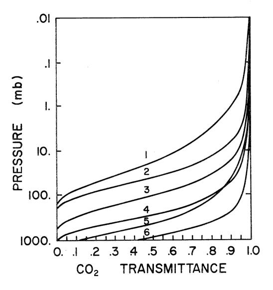
Figure 2. VTPR CO<sub>2</sub> Channel Transmittances for US Standard Atmosphere
