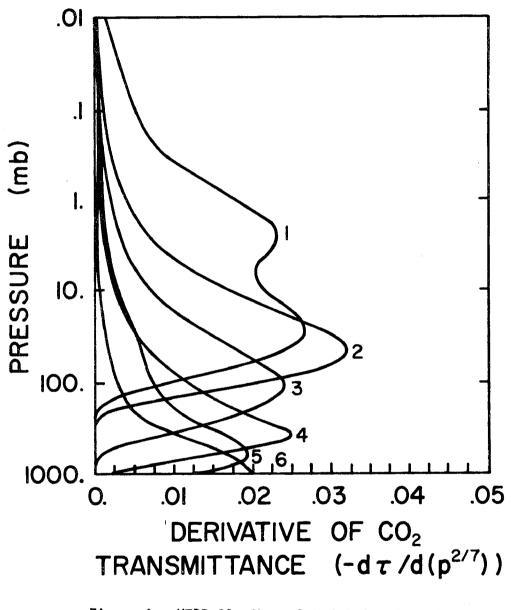
Figure 3. VTPR CO<sub>2</sub> Channel Weighting Functions for US <sup>2</sup> Standard Atmosphere
