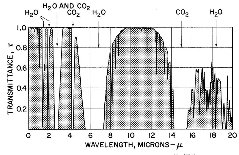
Figure 1. Infrared Transmission Spectrum (Hall, 1974)
