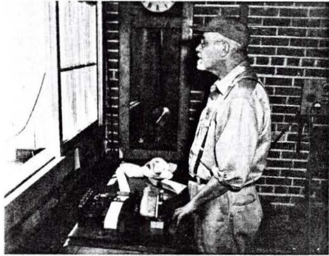
Fig. 3.5. Recording system for calibration of current meters, and tow car control switch. Strip chart records speed of tow car and revolutions per second of current meters.
