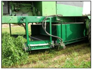
Fig. 2 Automated forage plot harvester used to harvest alfalfa plots at WCRC – Fruita. Photo by Calvin H. Pearson.
