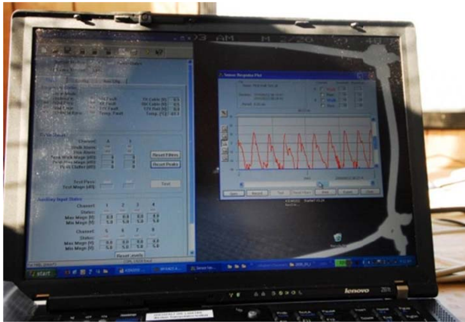
Figure 4.9: The Senstar Perimitrax® interface on a PC in the research trailer during a “walk” test by a human (Photo: Marcel Huijser, WTI/MSU).
