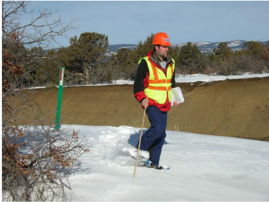
Figure 3.1: Example of a researcher crossing the buried EM cable. The green post in the background represents the location of the buried EM cable (cable extends left to right in photo). Tracks left in the snow by the researcher indicate the nature of the crossing activity by the researcher: perpendicular to the buried EM cable.
