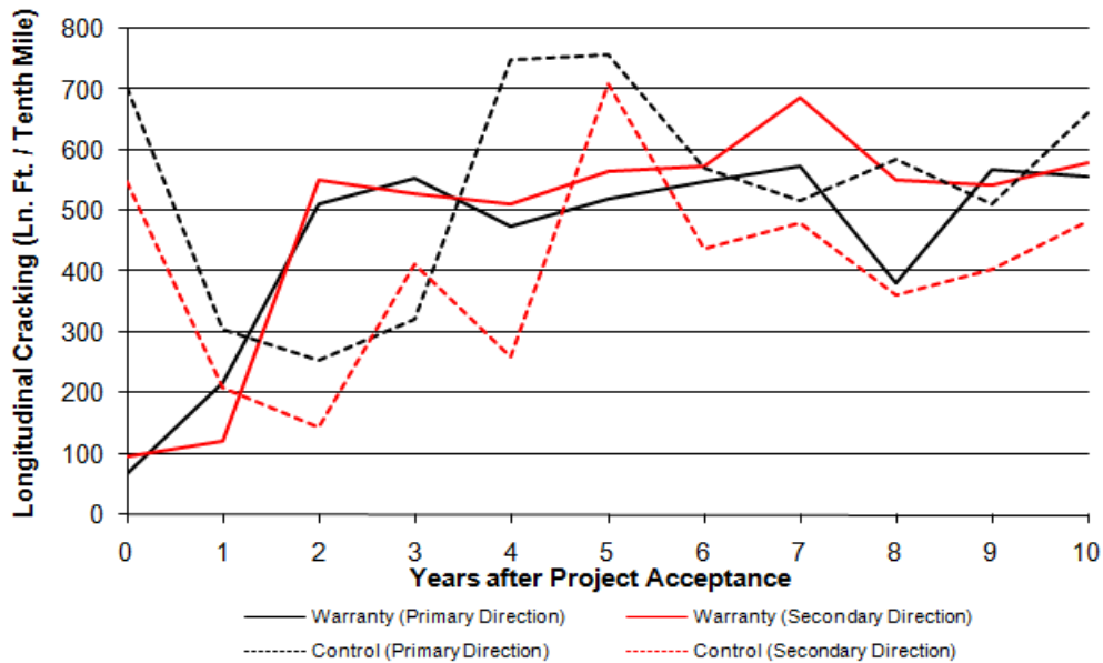
Figure 25. Comparison of the US 36/ I-76 longitudinal cracking performance
