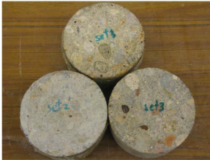
Fig. 2.1 RCC specimens for Rapid Chloride Permeability Test
