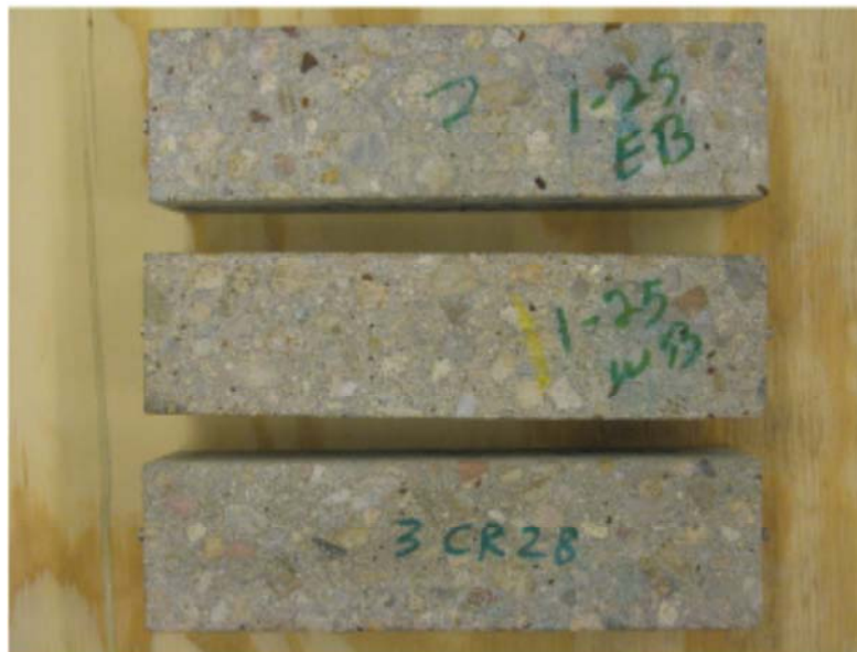
Fig. 2.3 RCC specimens for Drying Shrinkage Test
