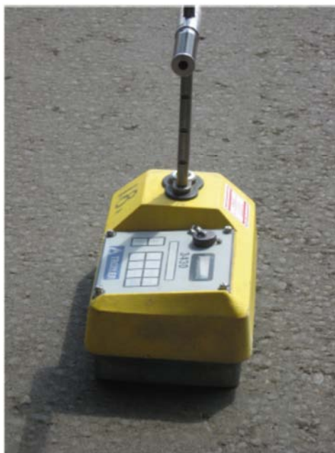
Fig. 1.8 A Nuclear gauge for measuring the degree of compaction of RCC pavement
