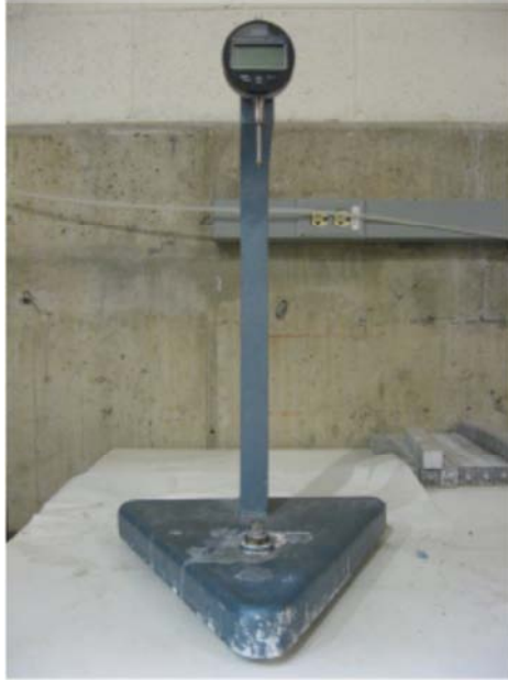
Fig. 2.4 A comparator for measurement of length change
