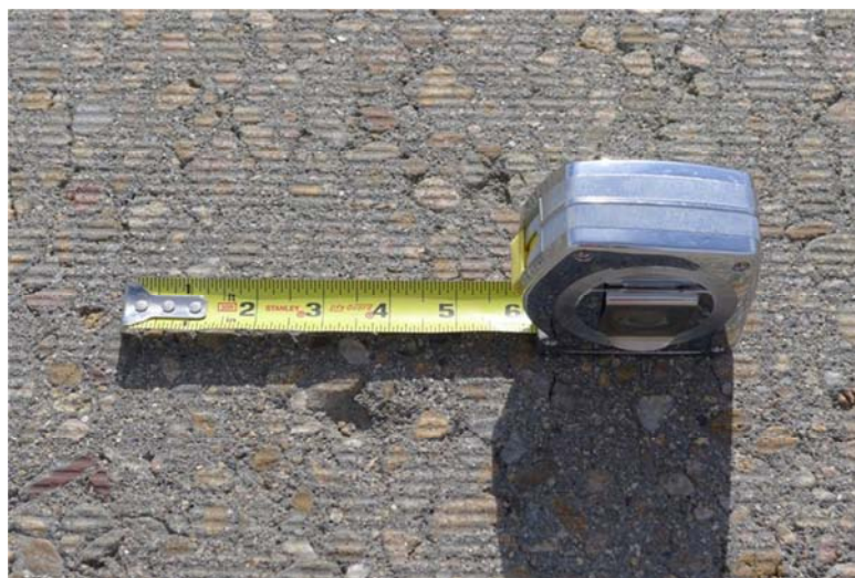
Fig. 3.13 A close-up view of the surface texture of the pavement at EB 66
