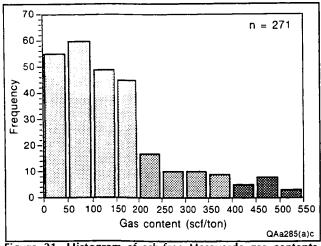
Figure 31. Histogram of ash-free Mesaverde gas contents. Most gas contents are less than 200 scf/ton (6.3 m<sup>3</sup>/t) but locally exceed 400 scf/ton (12.5 m<sup>3</sup>/t) in some coal beds.
