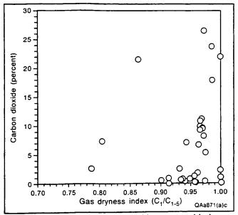
Figure 37. Variation of carbon dioxide content with the gas dryness index ( $C_1/C_{1.5}$  values). Coals with the higher carbon dioxide content generally have very dry gases, although coals in the Morgan Federal 12-12 and Colorado State 1-31 wells have wet gases.
