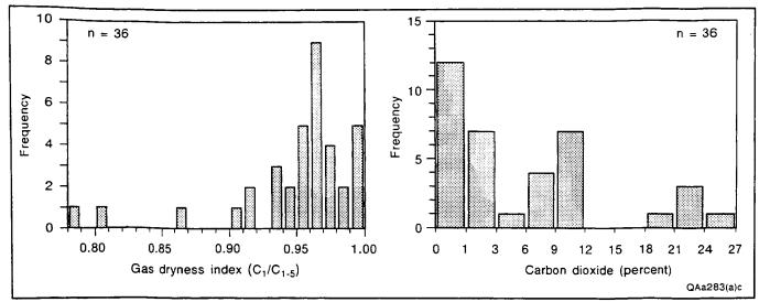
Figure 36. Composition of Mesaverde coalbed gases. Desorbed gases have a wide range of chemical compositions. Coal beds have entered the early gas generation stage as indicated by the minor amounts of wet gases in the samples. High carbon-dioxide contents in some coal beds may reflect bacterial activity, gas migration, and/or variations in maceral composition.
