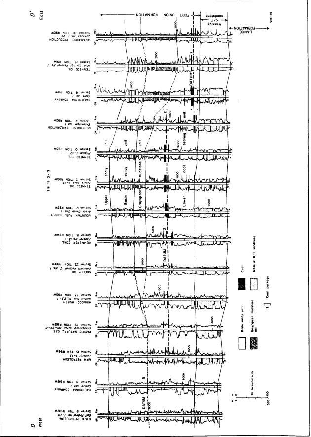
Figure 57. Detailed west-east stratigraphic cross section D–D' through T12N of the lower coal-bearing unit, Paleocene Fort Union Formation, Sand Wash Basin, illustrating occurrence of coal packages 1 and 2.
