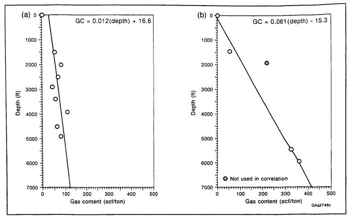
Figure 78. Gas content profiles and equations used for in-place gas and coal resource calculations. A moving average of 1,000 ft (305 m) intervals with 500 ft (153 m) overlap was used to determine a general relation between gas content and depth for the (a) Fort Union and (b) Williams Fork Formations.
