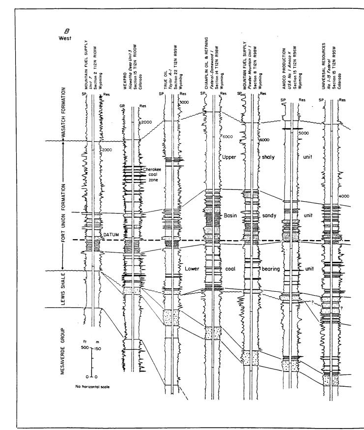
Figure 50. West-east stratigraphic cross section B-B' through T12N of the Paleocene Fort Union Formation, Sand Wash Basin, illustrating operationally defined stratigraphic units
