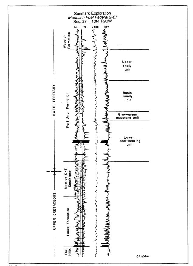
Figure 48. Type log and stratigraphic nomenclature of the Paleocene Fort Union Formation, Sand Wash Basin, and the occurrence of coal. Coal beds identified from density and sonic logs. See figure 52 for location.
