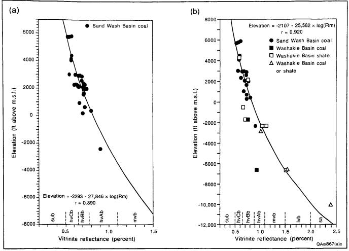
Figure 28. Vitrinite reflectance profiles, Sand Wash Basin. (a) Elevation versus vitrinite reflectance values of Mesaverde coals in the Sand Wash Basin. (b) Elevation versus vitrinite reflectance values of Mesaverde coals and shales from the Sand Wash and Washakie Basins. The equations in (a) and (b) were used to estimate vitrinite reflectance values based on depth in the two basins.
