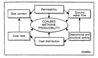
Figure 82. Interplay of geologic and hydrologic controls governs the producibility of coalbed methane.
