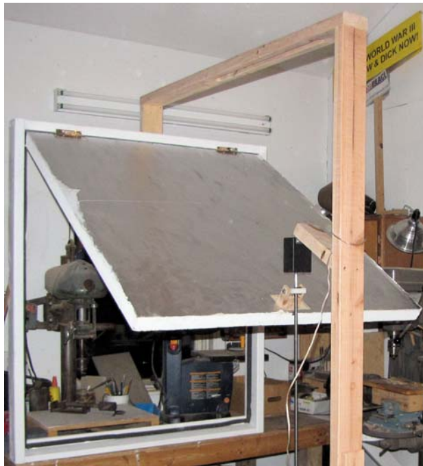
Figure 11. This lab prototype allowed the far end of the drive shaft to move through an arc of its own.
