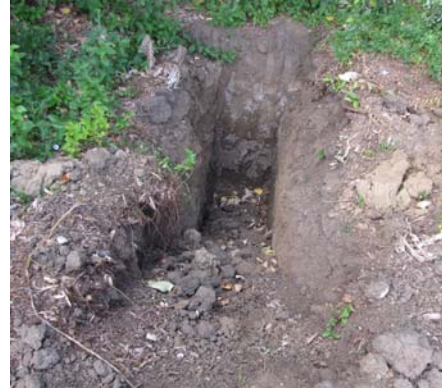
Figure 16. First four foot hole 16 days after digging is completely dry.
