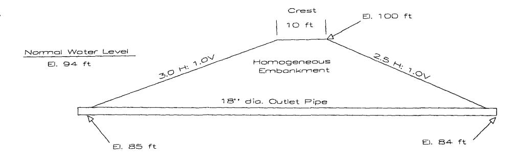
Figure 4 Mattie Dam and Reservoir Embankment Looking Upstream
