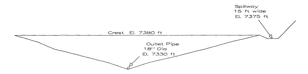
Figure 4 Currier Dam and Reservoir Cross Section at Outlet Pipe
