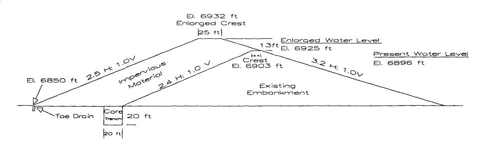
Figure 4 Red Mesa Dam and Reservoir Embankment Looking Upstream
