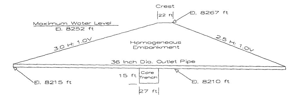
Figure 4 Sams Knob Dam and Reservoir Cross Section at Dam Center Line
