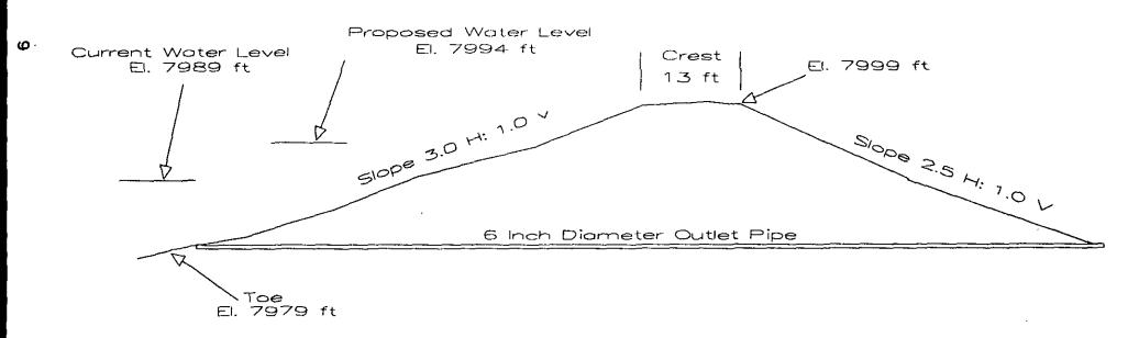
Figure 4 Palisade #1 Dam and Reservoir Cross Section at Dam Center Lind
