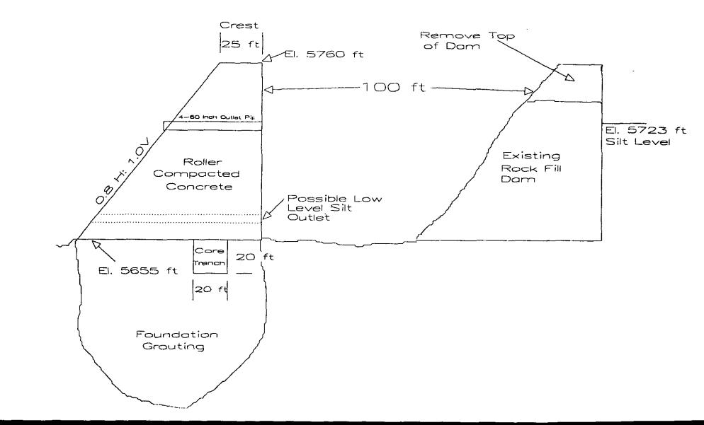
Figure 4 Cucharas Dam and Reservoir Cross Section at Dam Center Line Looking Upstream
