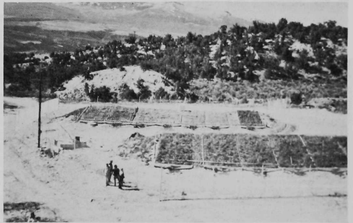
FIGURE 11 shows test plots constructed by Colorado State University near Anvil Points as part of a Federal- State- and industry- funded research project, "Rehabilitation and Revegetation of Spent Shale and Distrubed Lands." Plots were constructed with north- and south-facing slopes and designed to evaluate various plant species, shale treatments, irrigation techniques and runoff characteristics. The 7-ft
