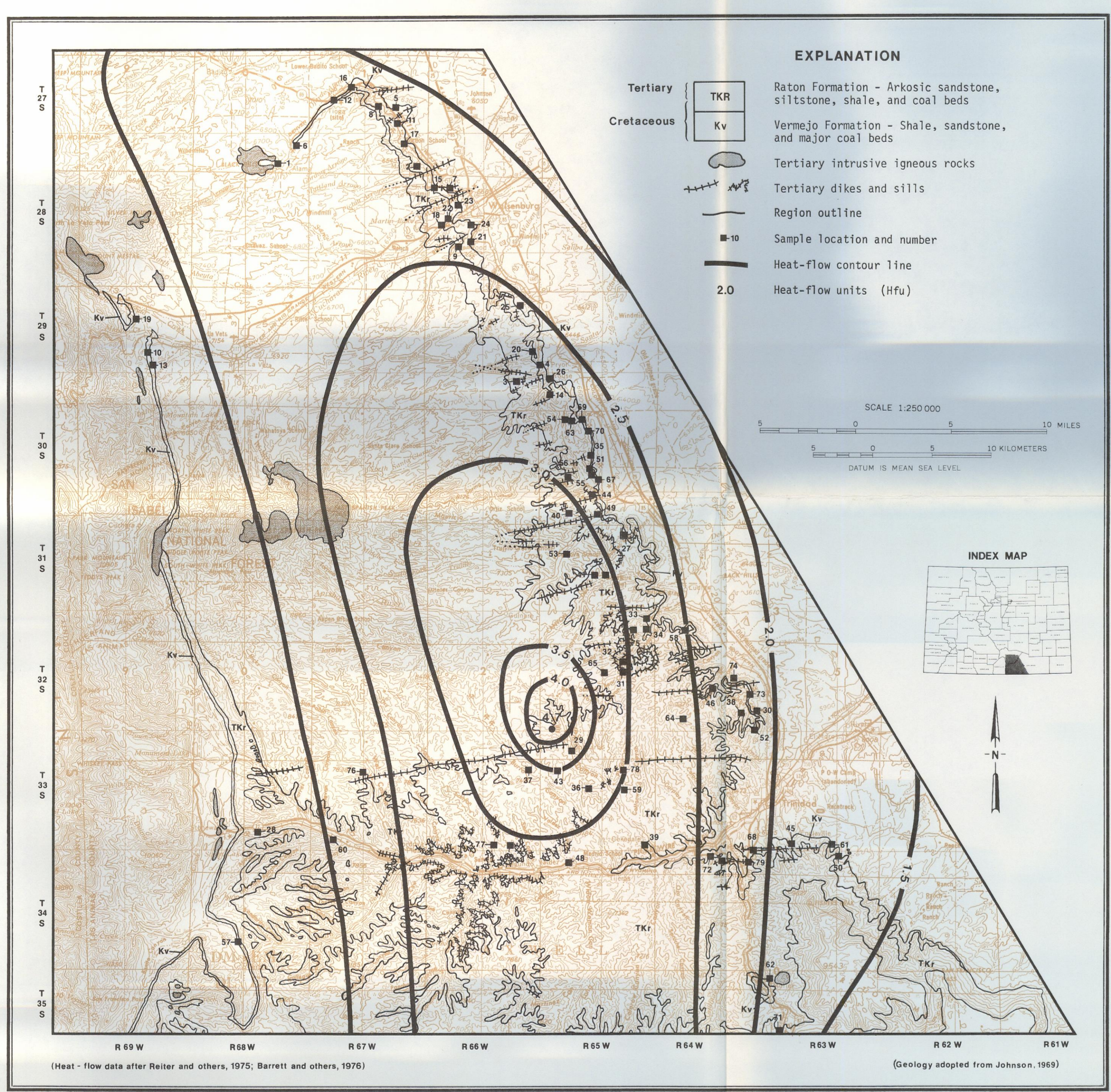
MAP A - COAL SAMPLE LOCATION AND HEAT FLOW MAP OF THE RATON MESA COAL REGION
