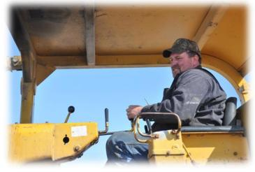
Lambrecht operates a piece of equipment called a skidder. A skidder has a grapple or cables that lift the trunks of several cut trees off the ground and drag them from the stump to another location. The trees are piled and a separate piece of equipment removes limbs and cuts the trunks to specific lengths. He is also the yarder operator and runs a suspended cable system that removes the cut trees when the terrain is too steep for a skidder.
