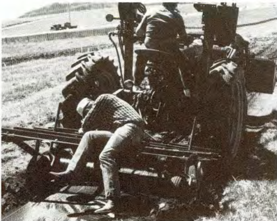
Weed barrier machine in operation. The person riding the machine cuts slits to pull seedlings through. Seedlings are planted before the weed barrier is put down.
