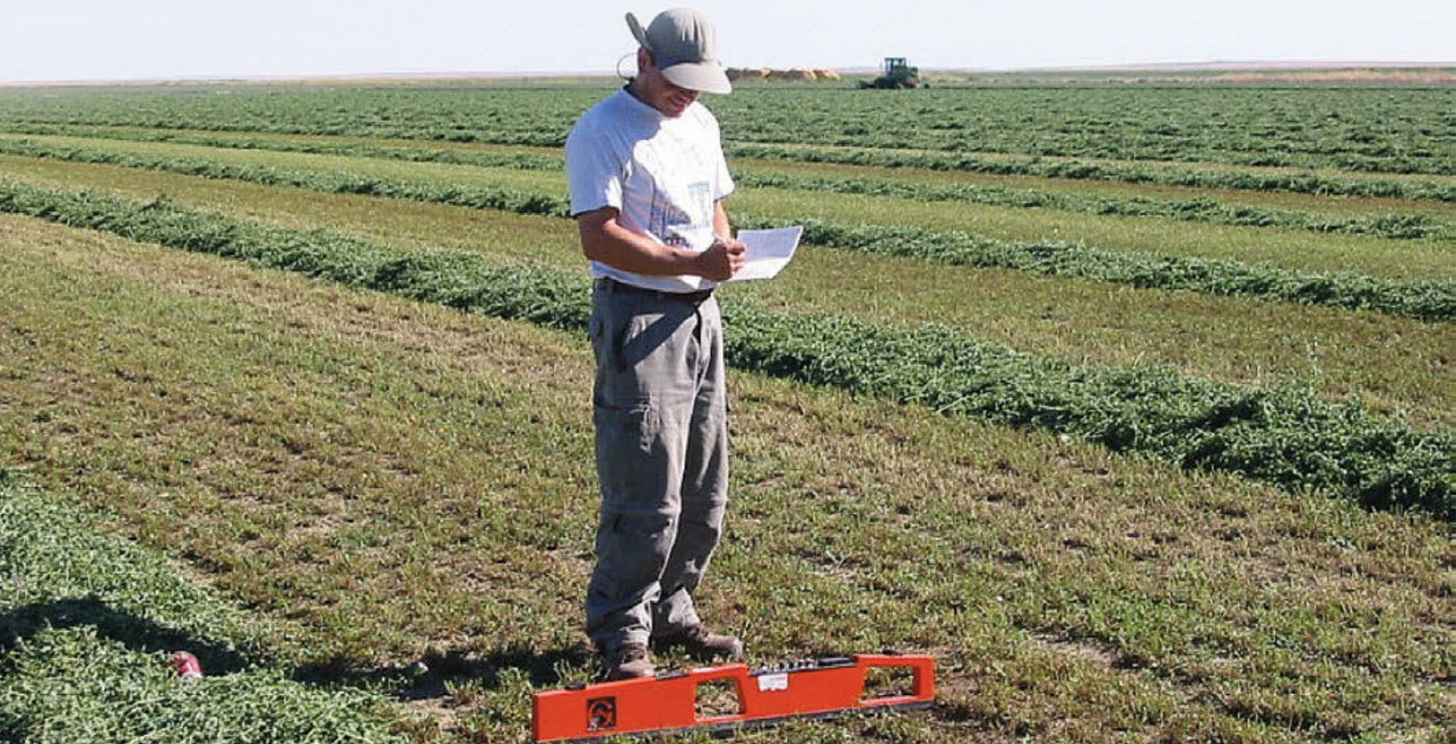
Figure 33. CSU technician conducting EM38 survey on a field in the LARV
