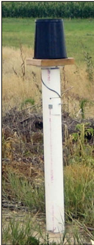
Figure 20. HOBO® rain gauge in Field US17E in 2008
