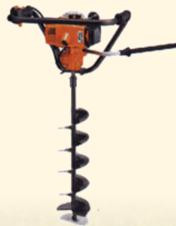
Figure 28. Stihl® gas-powered earth auger used for soil sampling
