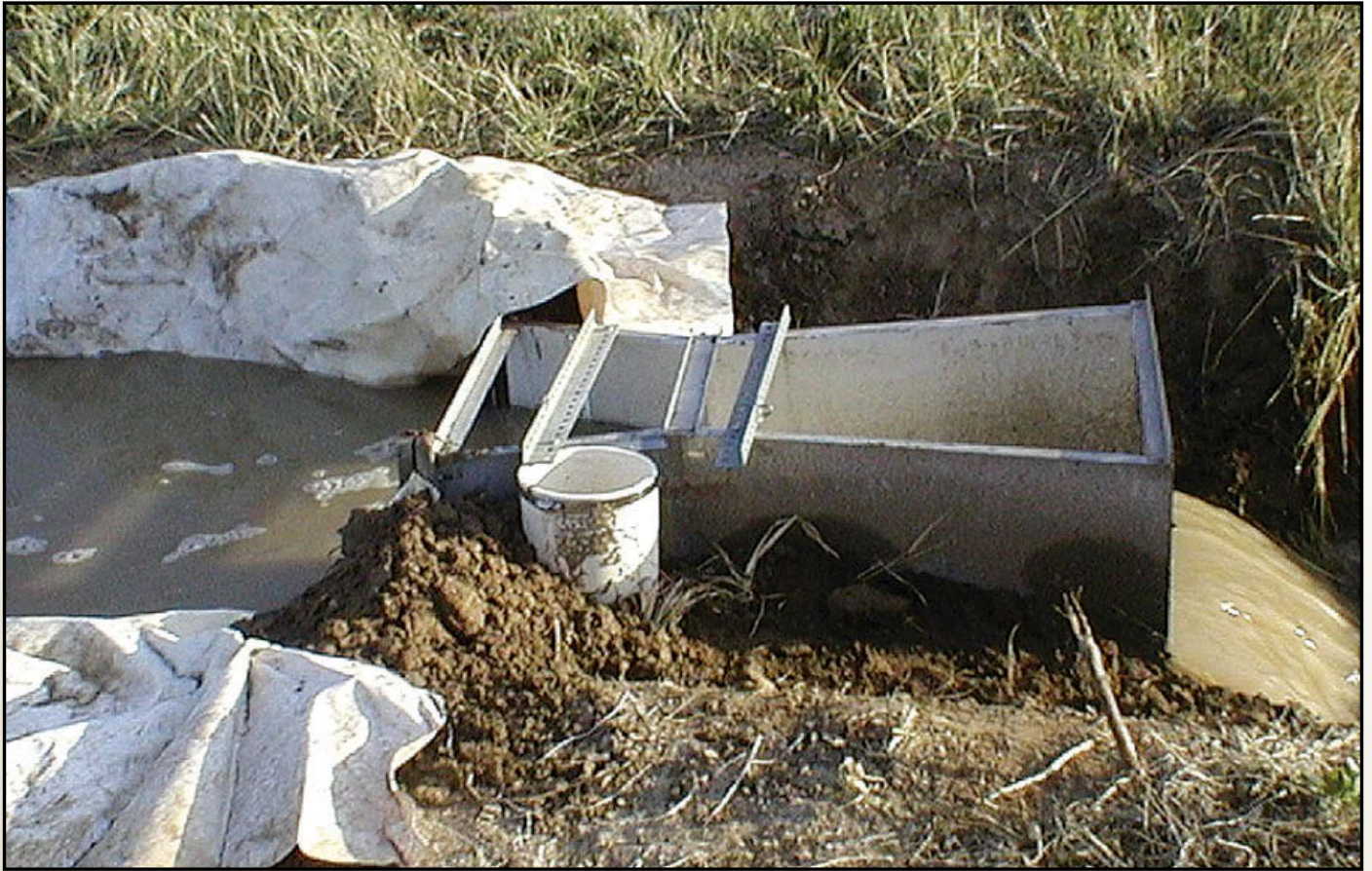
Figure 15. Cutthroat flume for measurement of tailwater runoff from field US14C in 2008
