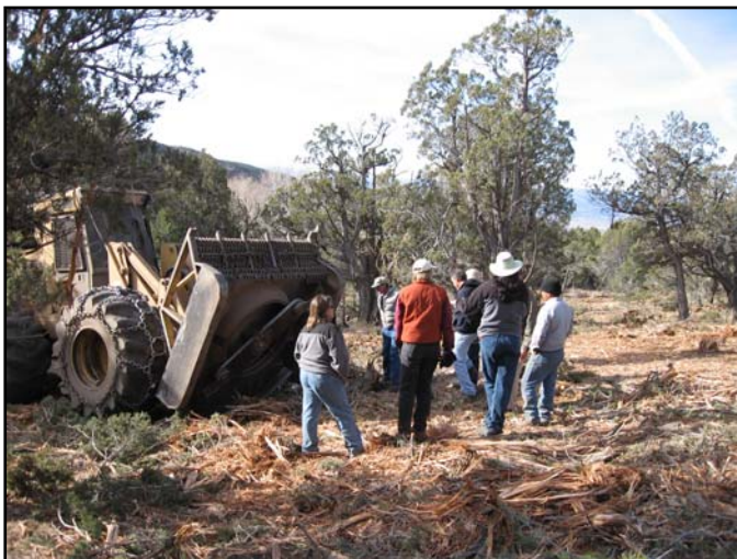
A hydro-axe is used to reduce fuel loads and improve the overall health of Grand Junction’s forest watershed.
