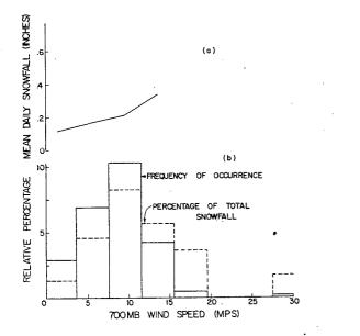
Figure 44. --(a) Mean Daily Snowfall at Wolf Creek Summit as a function of the 700 mb wind speed. (b) Distribution of total snowfall and total occurrences as a function of the 700 mb wind speed computed over a 4 mps class interval. realized per occurrence at the higher wind speeds.
