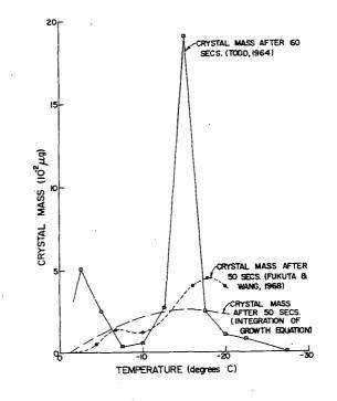
Figure 6. --Mass of a crystal after 50 to 60 seconds of growth as a function of environmental temperature.
