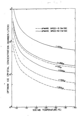
Figure 1. --Relationship of ice crystal concentration, ice crystal size, cloud top temperature, and vertical motion which optimizes the efficiency of cloud water utilization.
