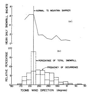
Figure 43. --(a) Mean Daily Snowfall at Wolf Creek Summit as a function of 700 mb wind direction. (b) Distributions of total snowfall and total occurrences as a function of the 700 mb wind direction computed over a 20-degree class interval.
