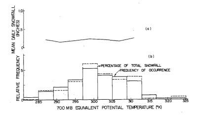
Figure 47. -- (a) Mean Daily Snowfall at Climax as a function of the 700 mb equivalent potential temperature. (b) Distribution of total snowfall and total occurrences as a function of the 700 mb equivalent potential temperature computed over a 4degree class interval.
