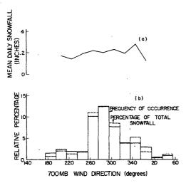
Figure 41. --(a) Mean Daily Snowfall at Climax as a function of the 700 mb wind direction. (b) Distributions of total snowfall and total occurrences as a function of the 700 mb wind direction computed over 20 degree class intervals.
