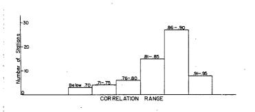
Figure 57. -- Snow water equivalent index vs. seasonal runoff, Colorado River Basin. No. of stations with indicated correlation coefficients in total of 70 stations.
