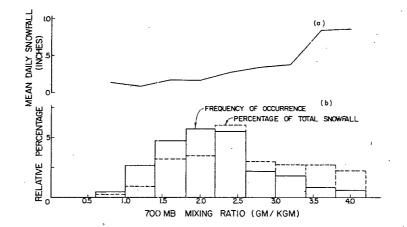
Figure 46.--(a) Mean Daily Snowfall at Wolf Creek Summit as a function of 700 mb mixing ratio. (b) Distribution of total snowfall and total occurrences as a function of the 700 mb mixing ratio computed over a .4 gm/kgm class interval.
