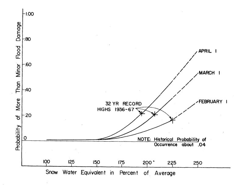
Figure 61. --Typical probability of more than minor flood damage for tributary streams to the San Juan during snow melt.
