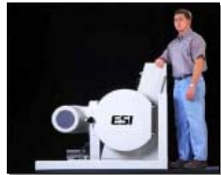
EB Curing Unit
