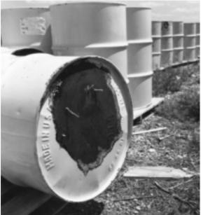
Barrels corroded and leaked plutonium-contaminated oil onto soil. Weeds grew through the badly corroded bottoms of these barrels.
