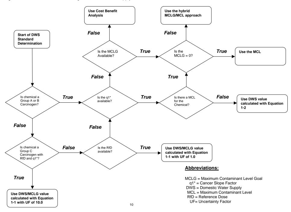
Figure 2. Flowchart for Determining Water+Fish Statewide Standards and Table Value Criteria.
