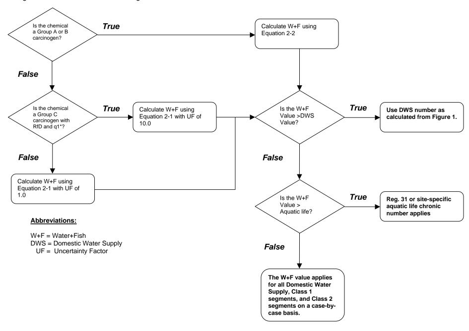
Figure 3. Flowchart for Determining Fish Ingestion Statewide Standards and Table Value Criteria.
