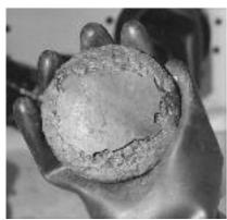
The plant produced weapons triggers or "pits" from plutonium buttons, pictured above.
