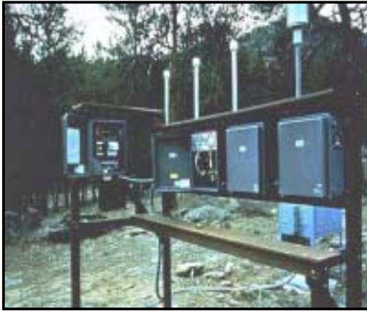
Fig. 2.0 Modular Aerosol Sampler, used for representation of physical properties of ambient atmospheric aerosols, including their concentration, and chemical composition
