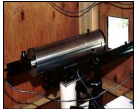
Fig. 2.2 Optec LPV2 transmissometer, which measures the ability of the atmosphere to transmit light. Two primary components: a light source (transmitter), and a light detector (receiver).
