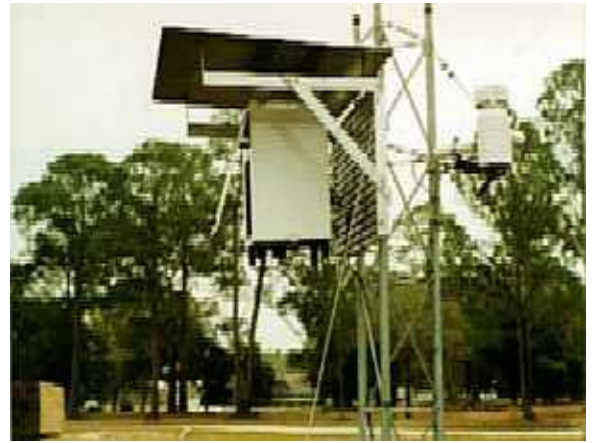
Fig. 2.1 Optec NGN-2 integrating nephelometer, used to estimate the atmospheric scattering coefficient ( b_{scat} ) by measuring light scattered by aerosols and gases in a sample air volume
