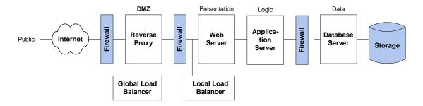
Figure 7.8.5 Three Firewall DMZ
