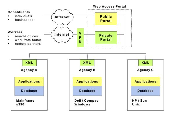
Figure 6.1 State of Colorado – Web Architecture
