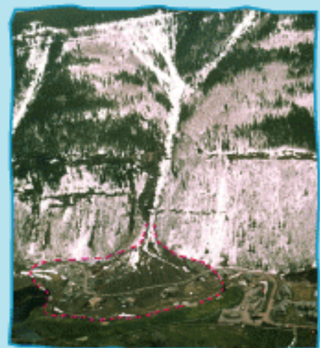
Avalanche zoning. These condos in Vail surround the runout zone of an avalanche path.
