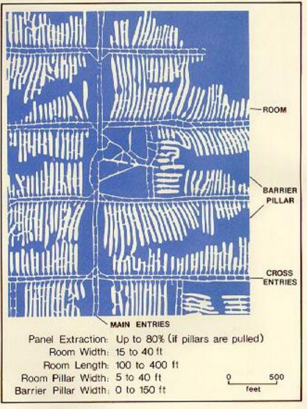
Figure 6a: The basic lay-out of a room and
