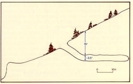
Figure 15. Cross-sectional view of an adit
