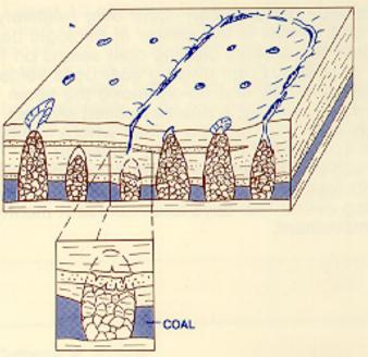
Figure 11. Block diagram of pit subsidence and trough
