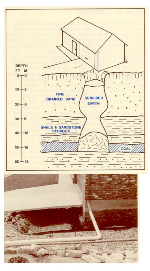
Figure 10. Cross section and photograph of a subsidence pit, under a house, in an area of thick soil cover. (*P.B. DuMontelle, 1981, Mine Subsidence in Illinois: Facts for the Homeowner, I.G.S., Environ.* Note 99. (photo by L. Floyd, Office of Surface Mining))
