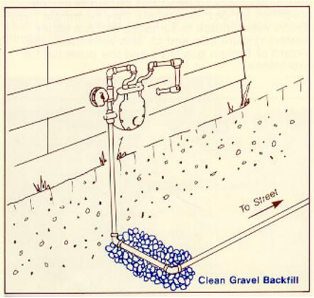
Figure 26c. Vented gas line outside of a
