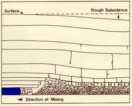
Figure 8. Cross-sectional view of a longwall
