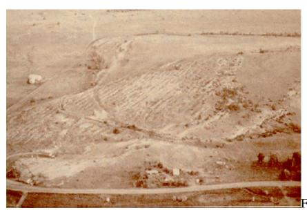
Figure 6b. Oblique aerial photo of subsidence over shallow mining in Boulder County, the location of rooms and pillars are visible in the outline.
