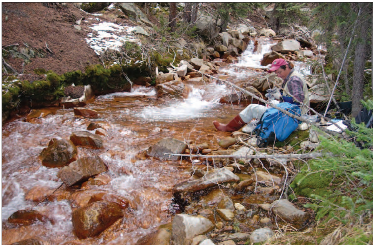
CGS field scientist samples a mountain stream to analyze for acidity and metals content. Note the red-orange color of the streambed due to the presence of iron oxide minerals—an indication of low pH and high dissolved metal concentrations. This stream may be impaired due to either naturally occurring conditions or acid mine drainage resulting from human activities. Photo by Bob Wood.
