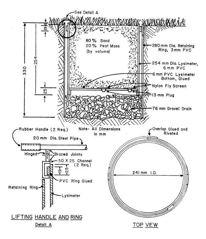
Figure 2. Schematic diagram of installed lysimeter and lifting handle.
